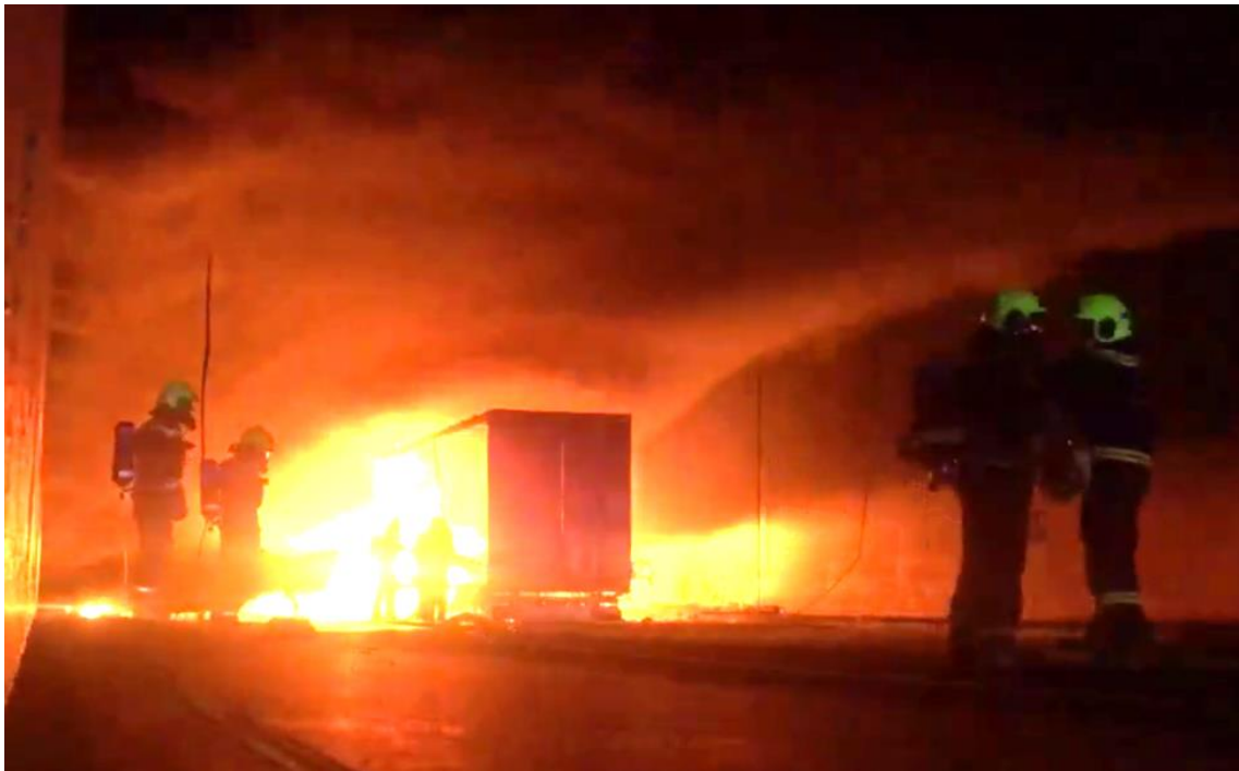
Figure 14: Firefighting an HGV Fire in a Highway Tunnel under Controlled Flow Conditions
